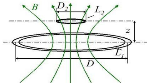
I found that some of the mobile phone makers are providing the wireless charging technology. However, the provided and the theoretical solution is not the same. The mobile phone manufacturers are providing a charging plate or a charging plate to charge the mobile phone. This charging mechanism is called as the inductively couples power transfer system.
